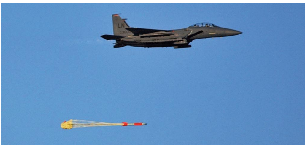
▲ In NATO's Steadfast Noon exercise, an F-15E fighter dropped a B61-4 nuclear bomb without live ammunition. Source: Sandia National Laboratory, USA
